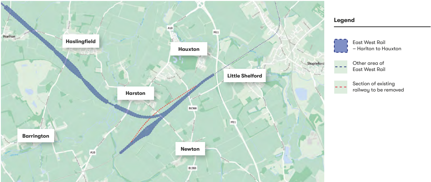
Figure 10.6: Offline construction: at-grade junction option
