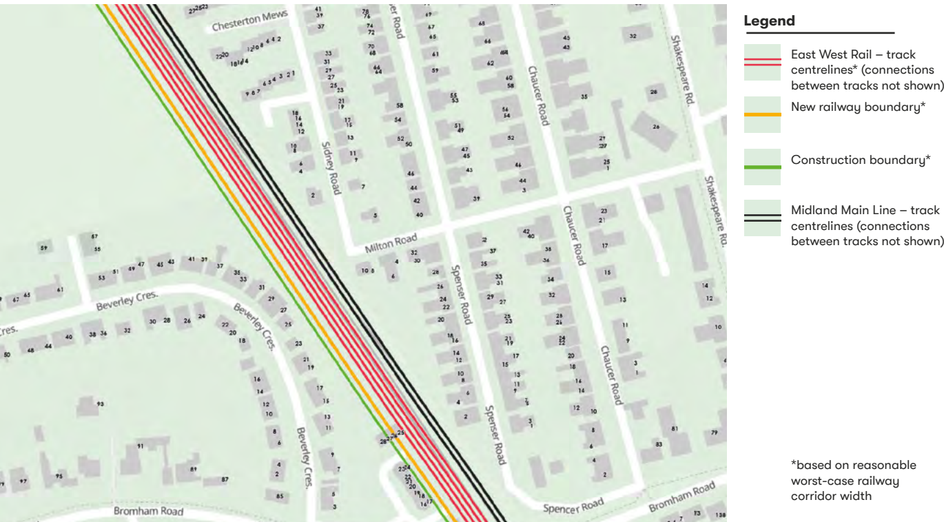
Figure 8.21: Six Track Western Variation B indicative track positions in reasonable worst-case railway corridor width
