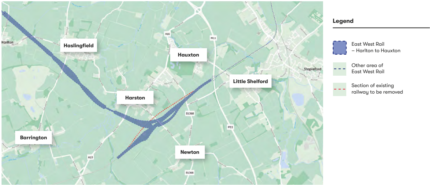
Figure 10.5: Offline construction: grade-separated junction option
