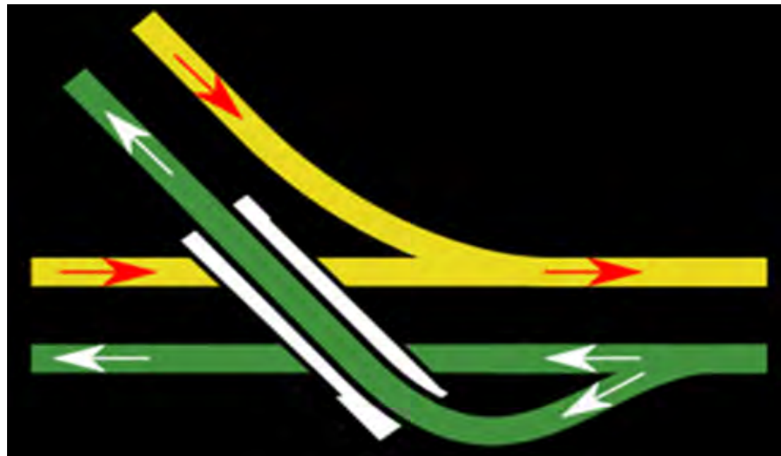
Figure 10.3: Typical grade-separated junction arrangement
