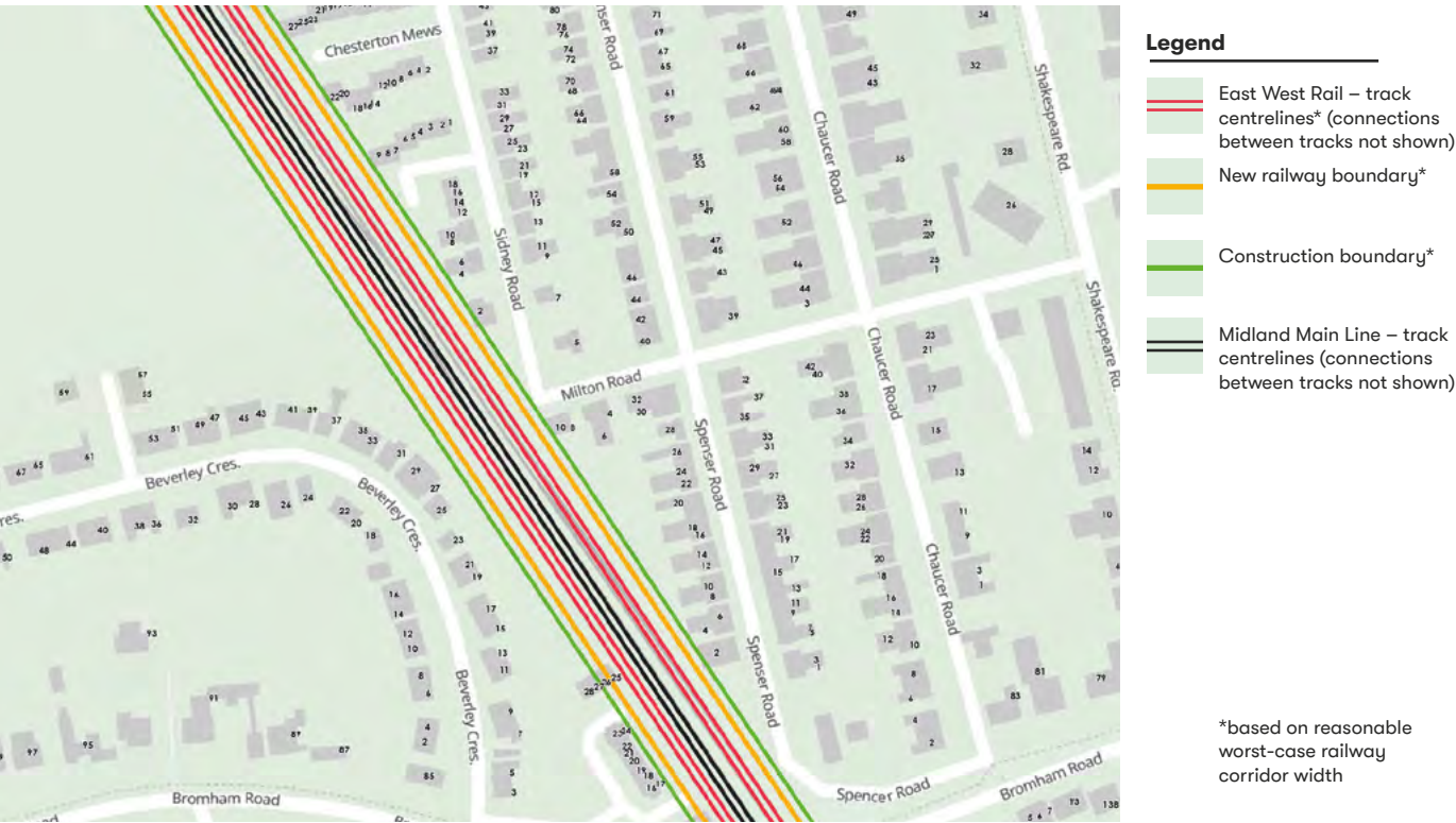
Figure 8.19: Six Track Western indicative track positions in reasonable worst-case railway corridor width
