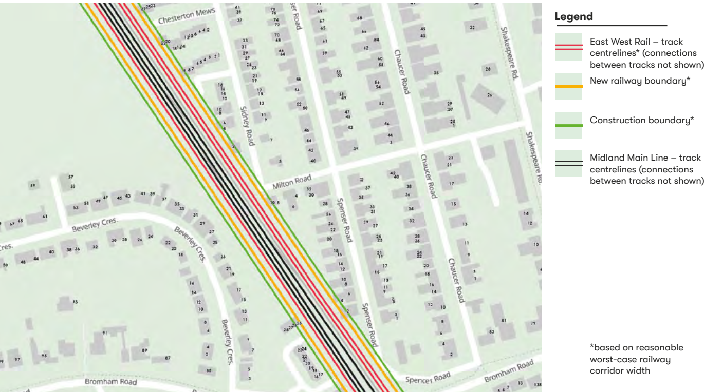
Figure 8.20: Six Track Western Variation A indicative track positions in reasonable worst-case railway corridor width
