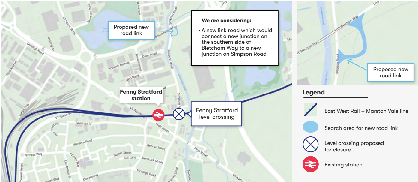
Figure 7.16: New link road between Simpson Road and H10 Bletcham Way (Vehicular Connectivity Option 2)
